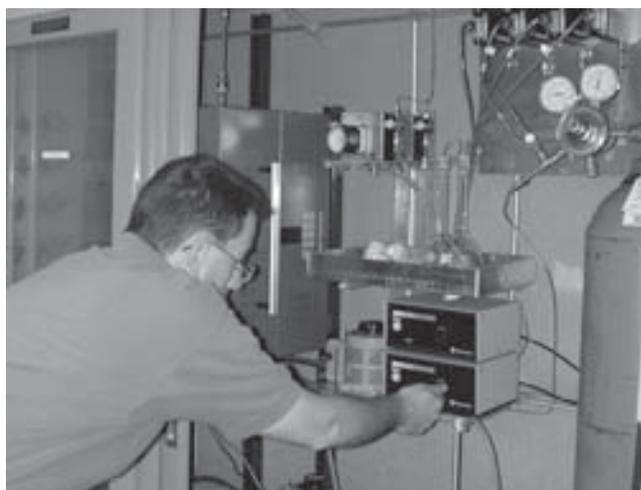
*Graduate student Andy Tadd adjusts the settings of the flow reactor for autothermal reforming of iso-octane (gasoline).*
