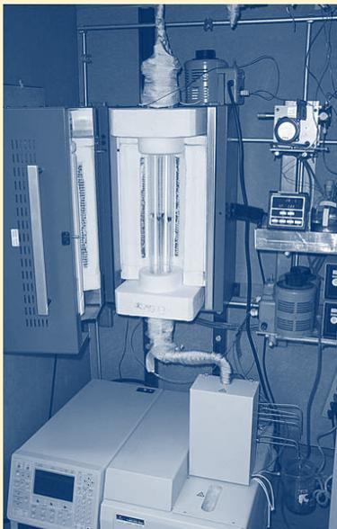
**Bench-scale fuel processing system in one of the TEC laboratories**
