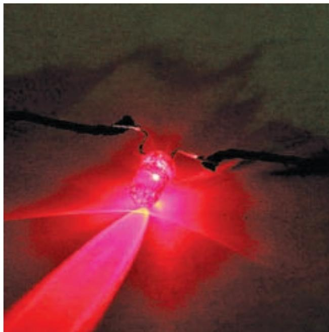
This carbon nanotube-coated smart yarn can conduct enough electricity from a battery to power a light-emitting diode device. Researchers can use its conductivity to design garments that detect blood.
